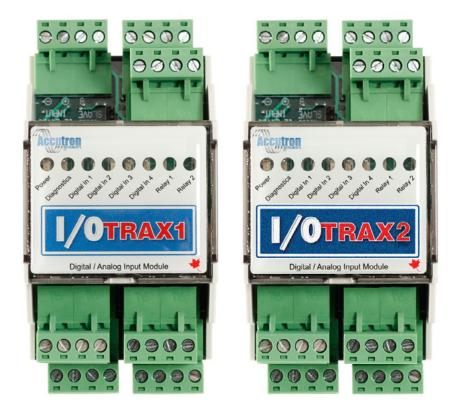
The I/O Trax system allows a users to install remote field I/O devices without having to invest in any other controllers. The I/O Trax is an affordable and practical distributed I/O system. This small modular device is easy to install to machinery or application components - saving time, troubleshooting, and excess field wiring.
