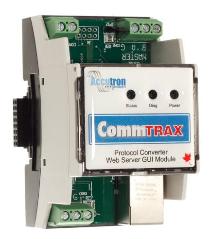
CommTRAX is a compact protocol converter that acts as a server, collecting data from various MODBUS RTU devices and distributing it at a low Bandwidth within a single register package.
