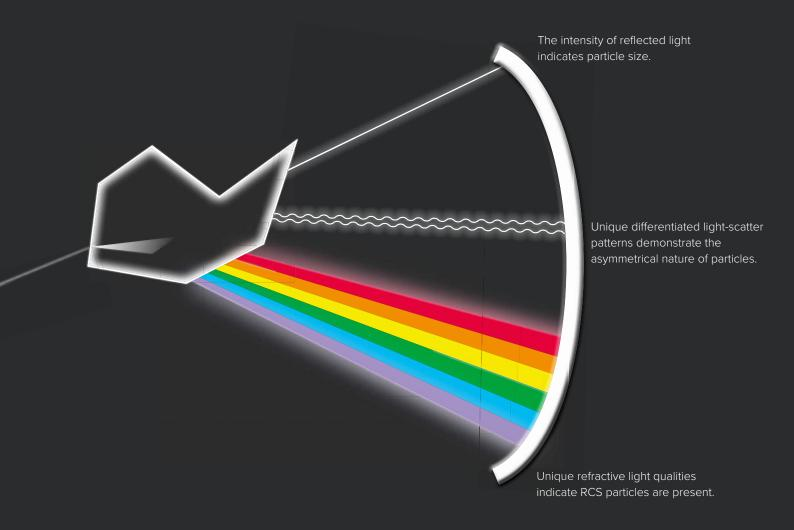
Our Breathe high-speed scatter/sizing/crystallinity detection algorithm processes the results in real time and triggers a triple-voting system that positively identifies and distinguishes harmful silica content.
