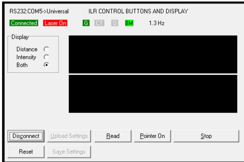
**System Configuration:** Data output format and selected ILR output data are displayed in the upper left corner. In this example the configuration is displayed as RS232:COM5.
